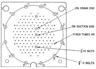
HEAD BOLT TIGHTENING SEQUENCE
